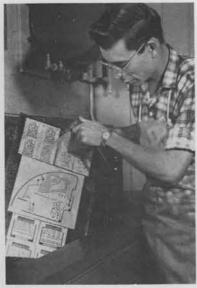
DEVELOPING the image on the laminate is performed by Kenny Anderson. Here he washes excess dve from the plate leaving only the exposed writing pattern visible on the copper.
